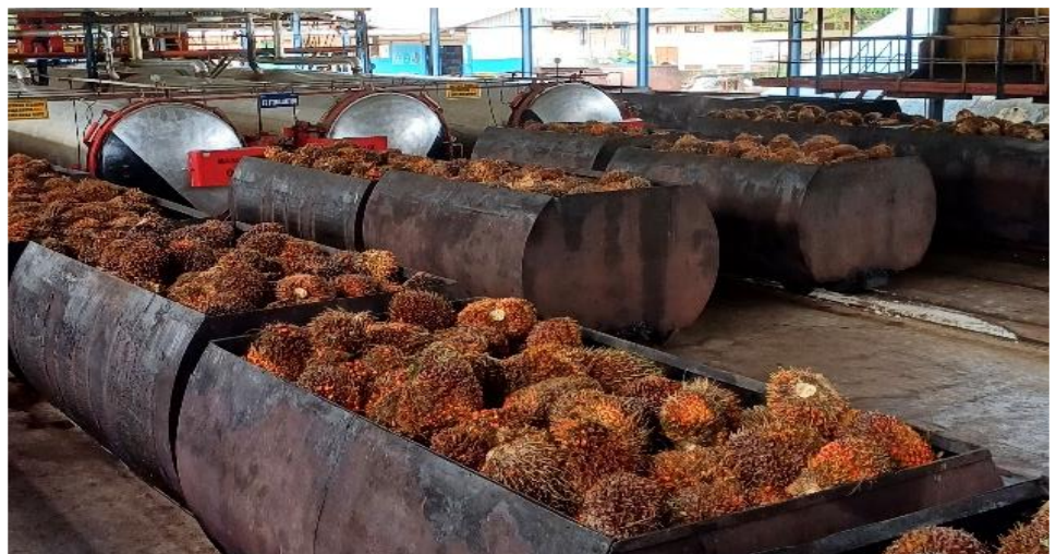
Figure 23. FFB sterilization process at SSMS's mill
